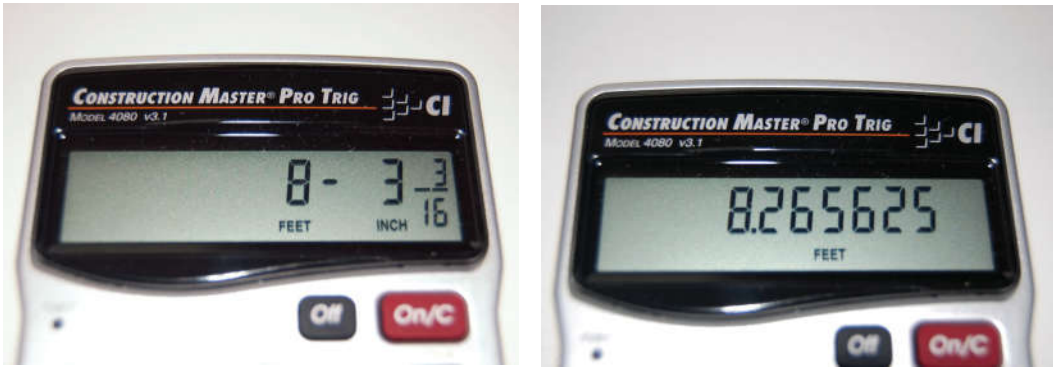
Figure 5.3 Construction Calculator Performing Conversions
