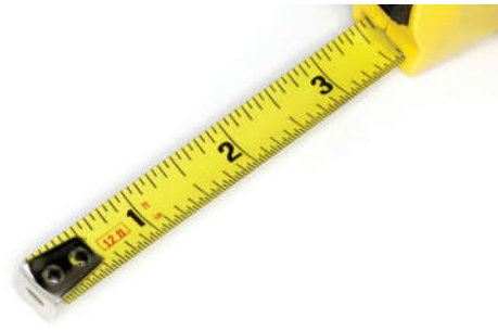
Figure 3.3 Tape Measure with Sixteenths and Thirty Seconds
