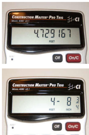
Figure 4.4 Construction Calculator Displaying Feet and Inches and the Decimal Equivalent
